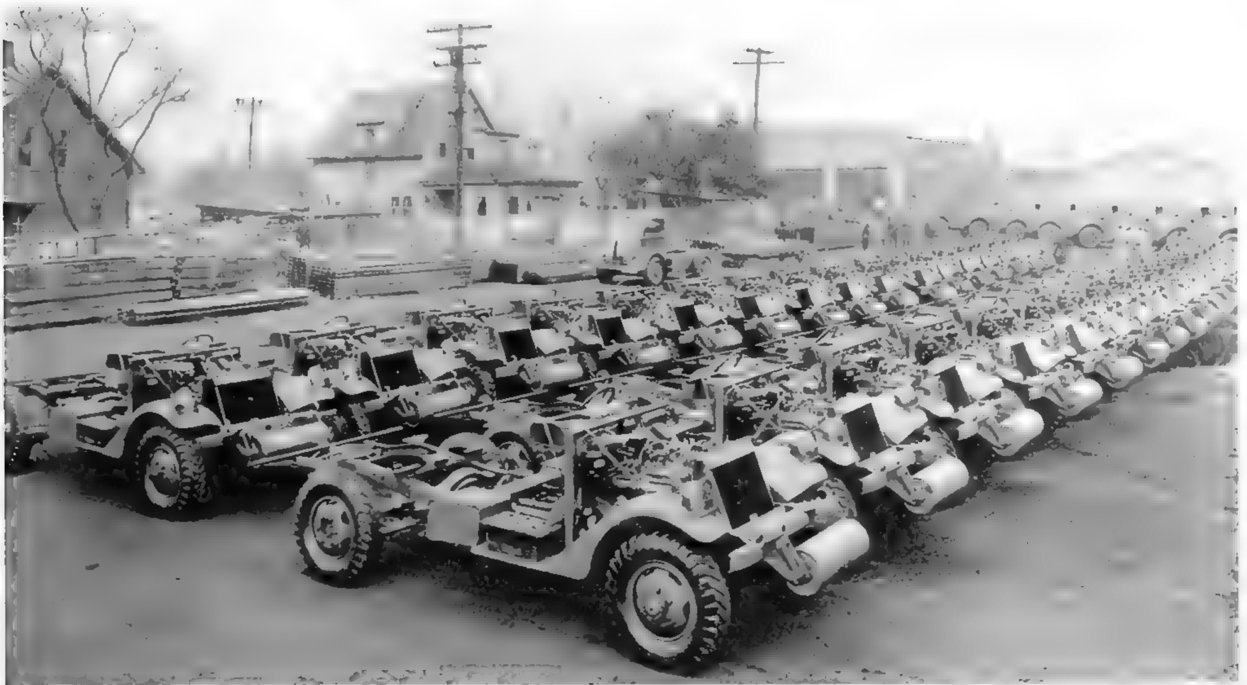
White assembled the M3A1 scout car chassis, but the armored body was installed by the Diebold Safe and Lock Co. These chassis, shown at White's Cleveland plant, await transport to Diebold's facility for this work. Notice the large Willard batteries installed, and the unusual tread pattern of the tires. (Photo courtesy of Diebold, Inc.)
